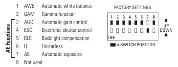
Figure 1. Switch Settings for Varifocal Lens
